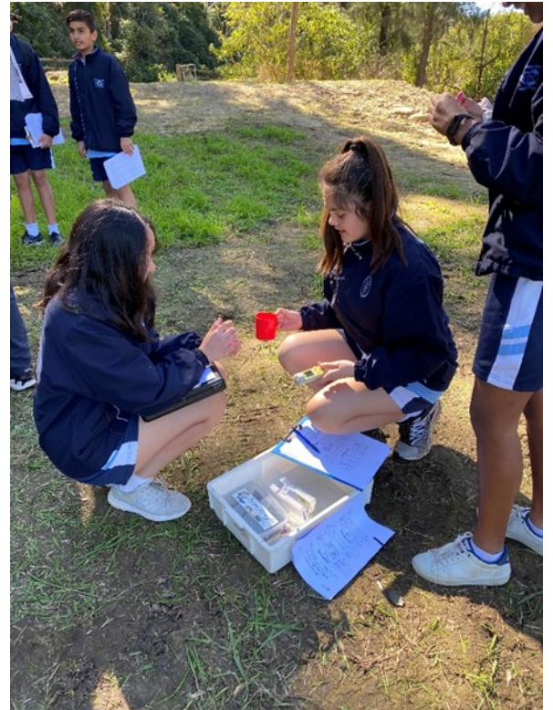
Using specialist equipment to test the water quality of the river.
