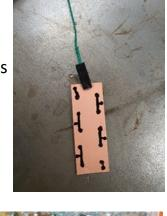
Students have also worked on the construction of a resistance bridge. This is an important project, as it gives the students the opportunity to etch copper PCB board and make their own circuit boards. The end product helps students calculate the value of
